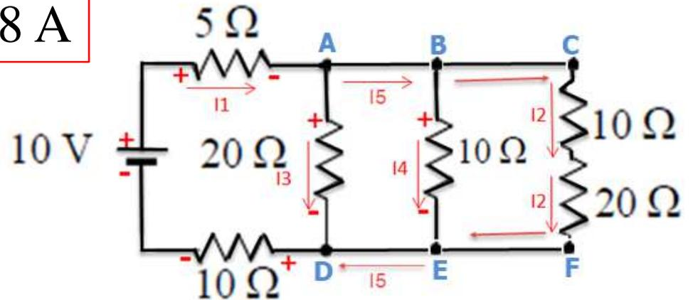
$$\Delta V_{CF} = V_C - V_F = 20\Omega \cdot I_2 + 10\Omega \cdot I_2 = 2,6596 \text{ V}$$
